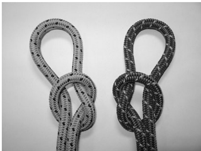
FIG. 3—Overhand slip loops, S (left) and Z (right).
