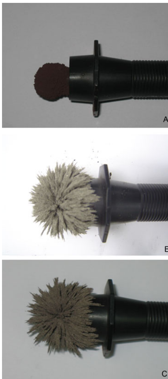
FIG. 3—(A) Weak attraction between the powdered magnetite and the magnetic applicator. (B) Strong attraction between the Ni powder and the magnetic applicator. (C) Strong attraction between the prepared powder and the magnetic applicator.
