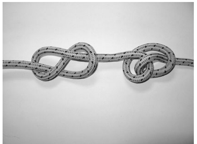
FIG. 12— Figure eight knot (left) and Pretzel knot (right).
